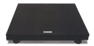
he DAB1 is made from a single sheet of 15mm black acrylic fitted with double-sided Delrin and absorbothane feet. Delrin is a hard acetal resin and absorbothane is extremely good at absorbing vibrations with excellent anti-slip properties. The only disadvantage is that it tends to stick firmly to any smooth surface, making it difficult to move the platform. However, this can be overcome by fitting to the exposed surface a disc of black paper, which adheres to the absorbothane but not the table!
